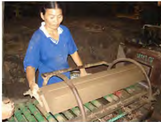
Extruder and wire cutter (stiff-mud process)
