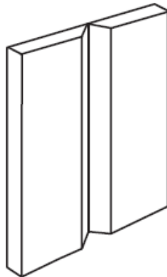
(C) VERTICAL WELDING TEST POSITION 3G
