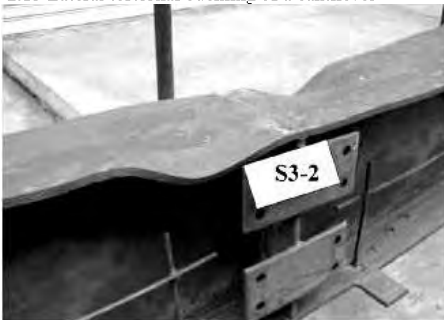
Figure 2.13 Lateral torsional buckling of a cantilever
